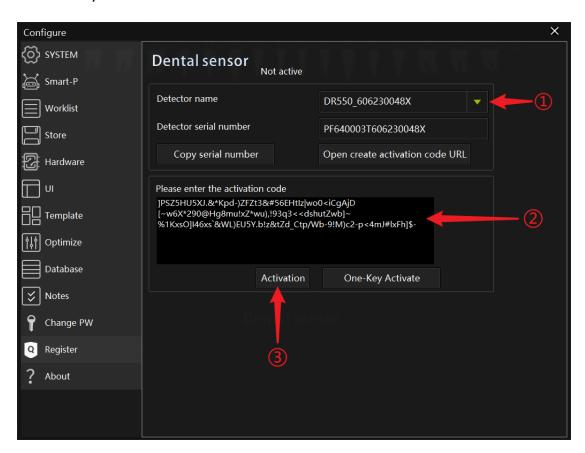
4. Here, the current probe registration ends, After the detector is activated successfully, the software needs to be restarted before use.
